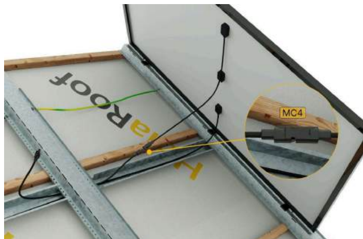
DC cables routed in metal channel; MC4 strain relief ensured before lowering the module.
